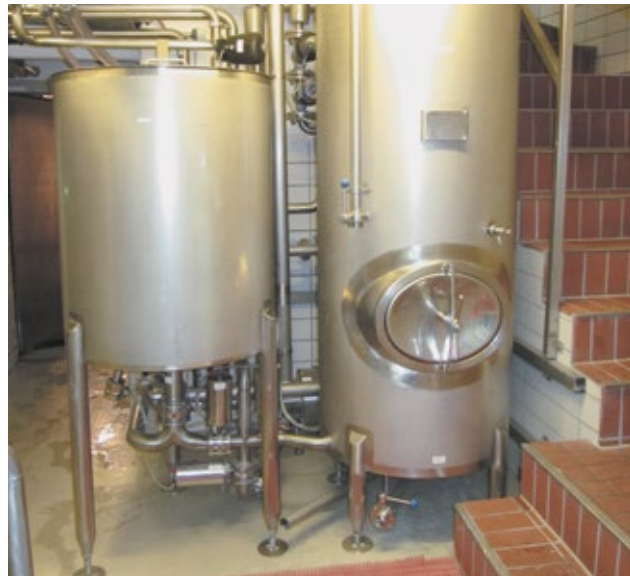
The innovative CIP plant leads to lower mixed phases of water and beer as well as to a clear reduction of the waste water load.
